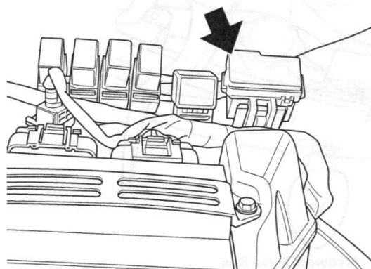
Arrowed: Fuse Box
